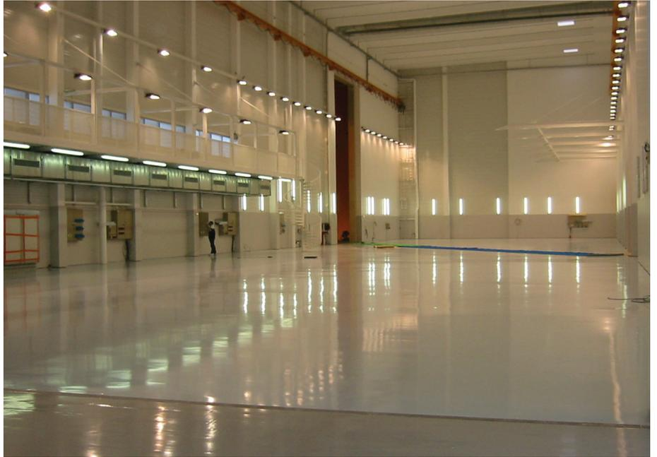
face for the product installation. The entire area was then covered with Stonclad GS, a troweled mortar base designed to provide durability and long-term protection against impact, abrasion, and heavy-duty traffic. Stonkote GS4, a general service epoxy coating, was applied to provide an impervious, chemical-resistant surface to withstand punishing aircraft fuels and oils. Stonclad's seamless finish allows easy cleanup of the harshest chemicals and keeps maintenance expenses to a minimum.
